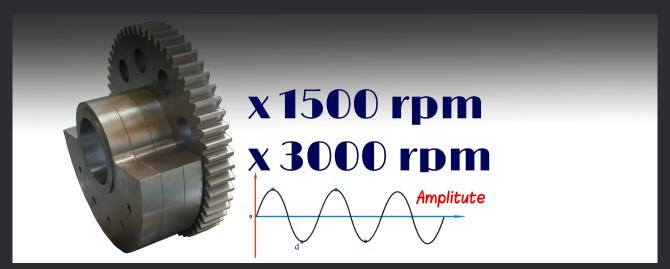
The ground formation and the eccentric moment with centrifugal force are the basic parameters of the driving process by vibratory hammers.
